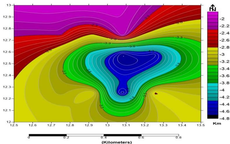
Fig. 6 2D spectral magnetic depth to basement contour map of the study area (contour interval 0.1).
