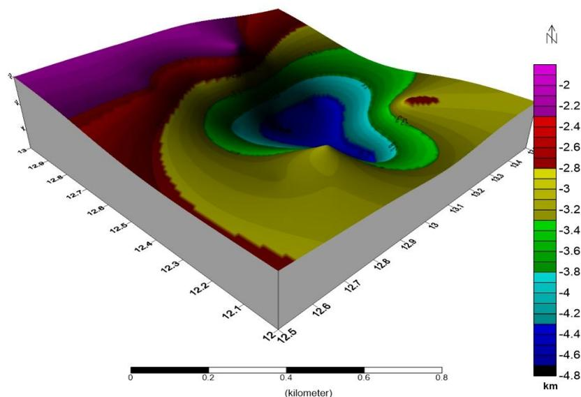
Fig. 7 3D surface map of magnetic depth to top of basement of the study area from spectral depths.
